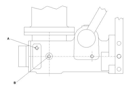
To check the gearbox oil level. Remove plugs A and B and check that the oil level is up to the level of the bottom of the threaded hole B. If not fill with Renogear V220EP through hole A until it flows from hole B. Replace plugs A and B.
