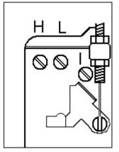
• Turn the idle speed adjusting screw (I) counter-clockwise until the drilling spindle stops rotating - then turn the screw approximately one half turn in the same direction.
